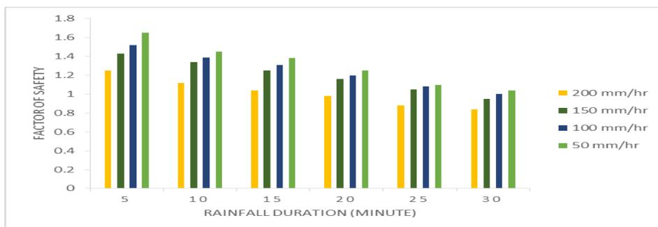
**Fig. 5 Factor of Safety of Slope Angle  $26.8^{\circ}$  with Vetiver Plant for different Rainfall Intensity and Duration.**
