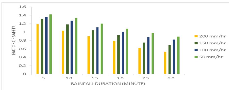
**Fig. 4 Factor of Safety of Model Slope Angle  $26.8^{\circ}$  without Vetiver Plant for different Intensity and Duration.**
