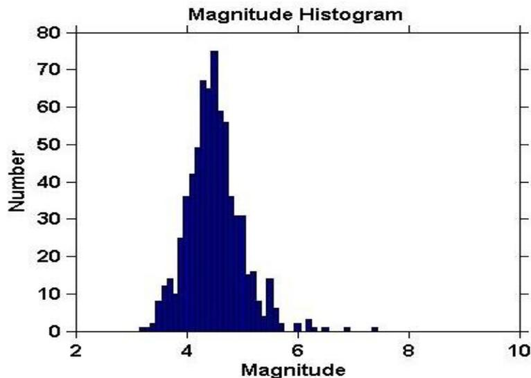
**Figure 2.** The magnitude-frequency curve of earthquakes in the study area
