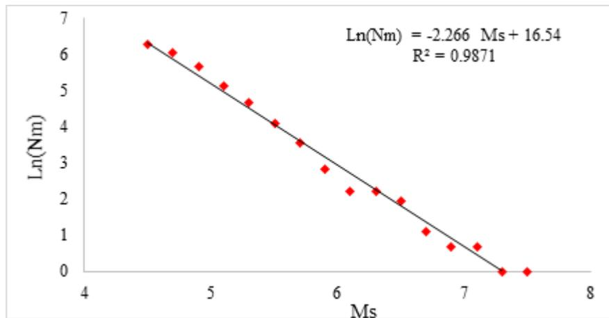
**Figure 7.** Gutenberg-Richter curve and calculation of seismic coefficients of  $\alpha$  and  $\beta$
