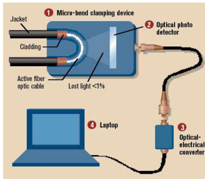
**Fig. 6. Optical Electro Converter**
