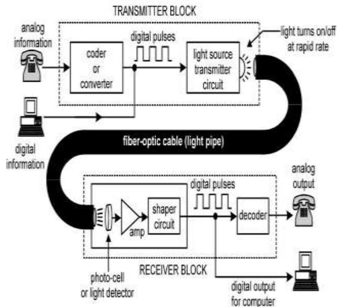
**Fig. 4. Fiber Optic Communication Block Diagram**
