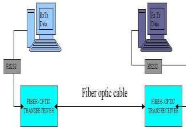
**Fig. 5. Fibre optics for PC to PC Communication.**
