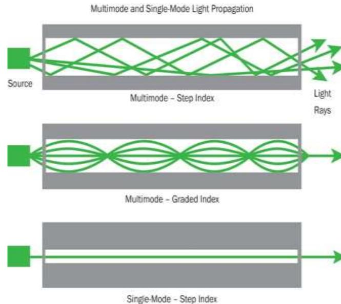
Fig. 2. Fiber Optics Mode. Source: Fiberopticshare.com
