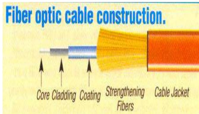
**Fig. 1. Fiber Optic cable Construction.**
