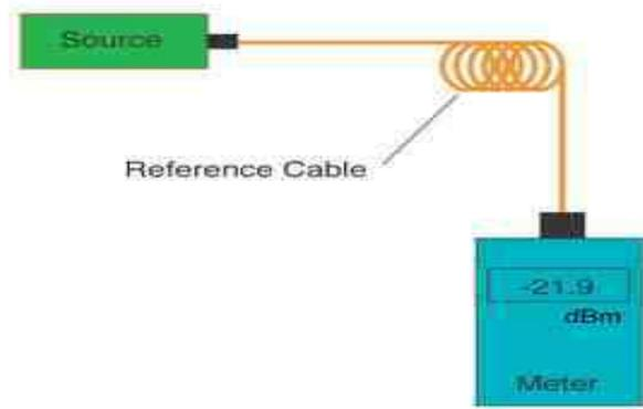
Fig. 7. Optical Power Meter . Source (FOA)
