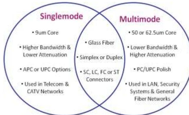
Fig. 3. Fiber Modes Comparison. Source: Cables-solution.com
