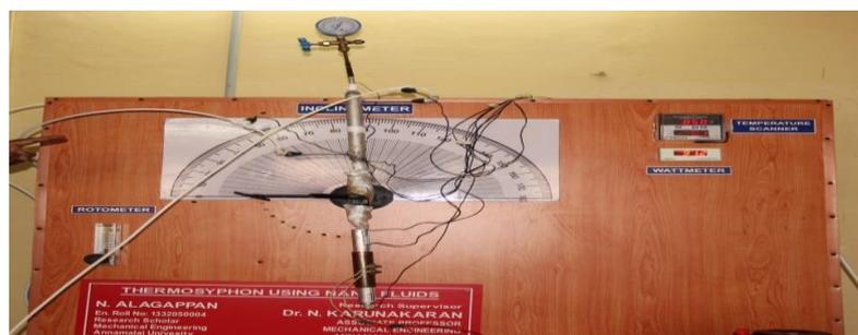
**Figure 3: Photographic View of Test Rig with 6063 AA TPCT**
