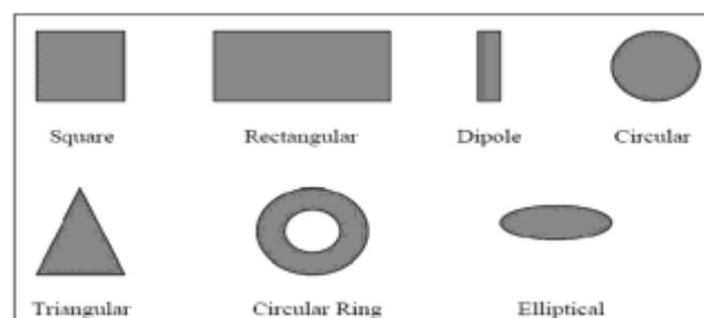
**Figure 1:** Different shapes of patches for antenna
