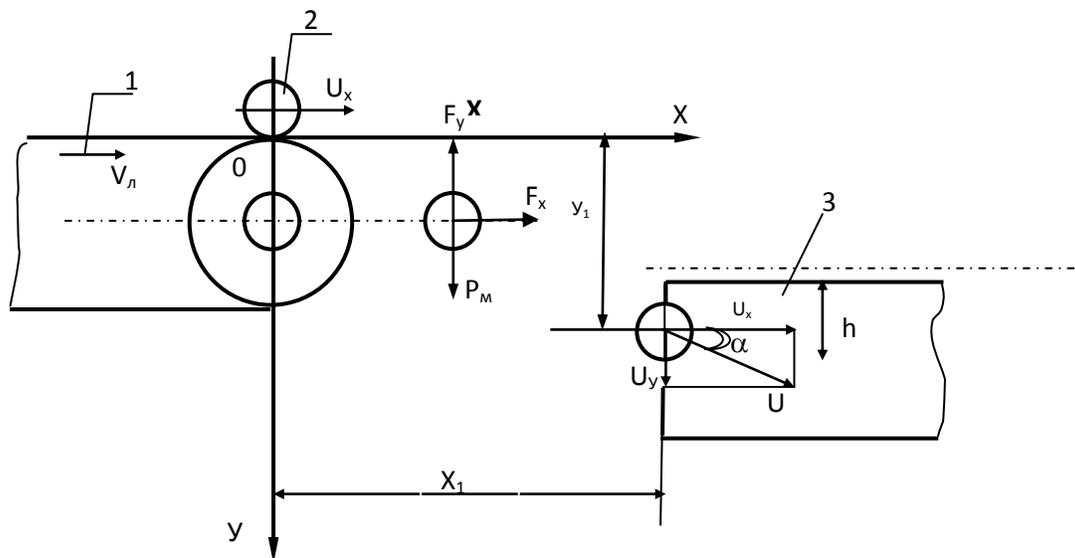
Picture 3: Transferring the Cotton to the Air Transporting Device through the Ribbon Device
