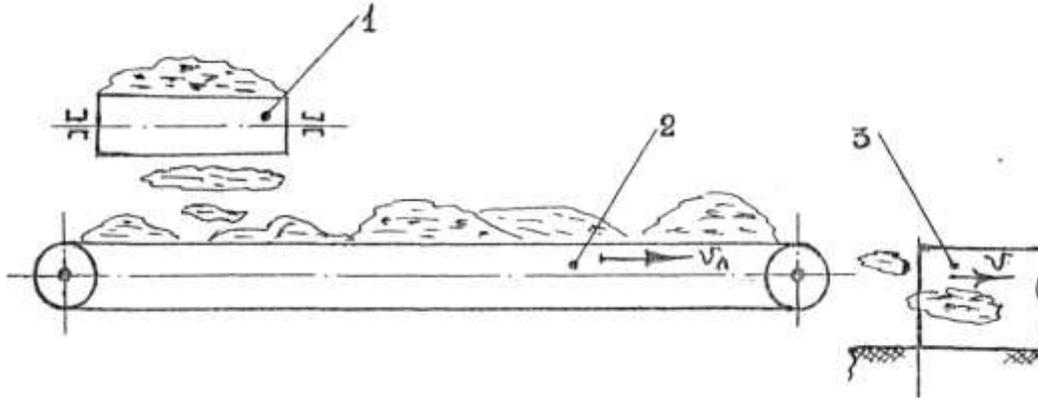
Picture 2: An Experimental Device Scheme Designed to Study the Non-conformity of Cotton Delivery
