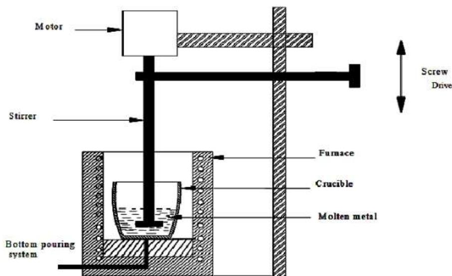
Figure 2: Aluminium Metal Matrixes Composite by Stir Casting Method
