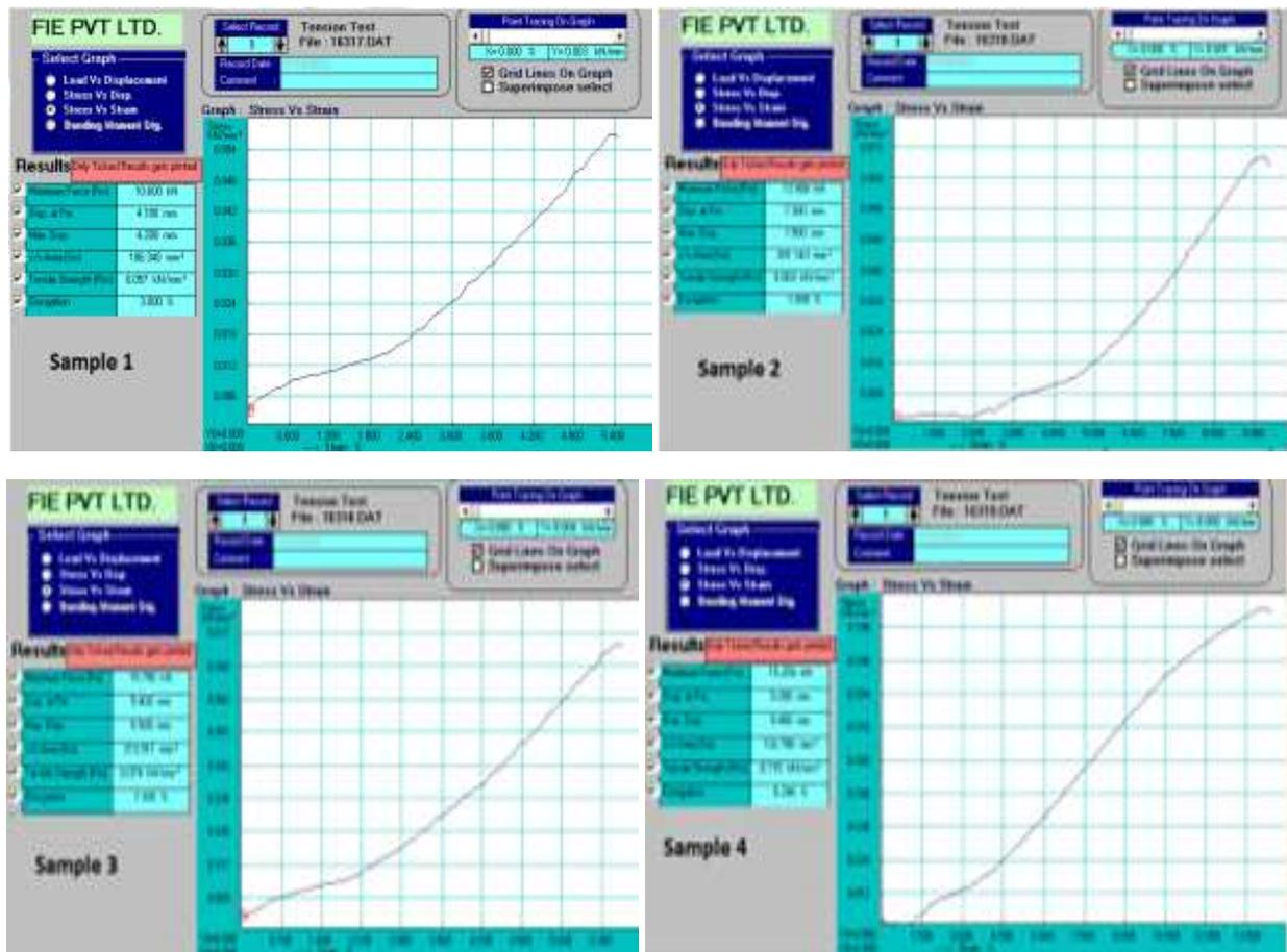
Graph 2: The Stress Strain Curves of different Samples
