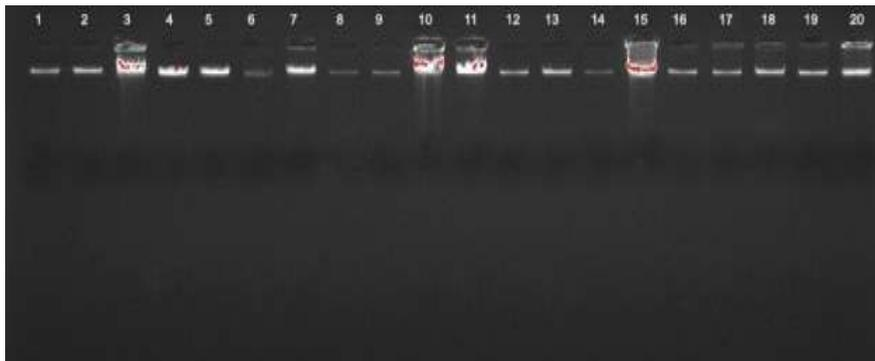
Fig. 1: Agarose Gel Electrophoresis of Bacterial Genomic DNA Using 0.7% Agarose, TBE (1x) and Visualized by Ethidium Bromide Stain
