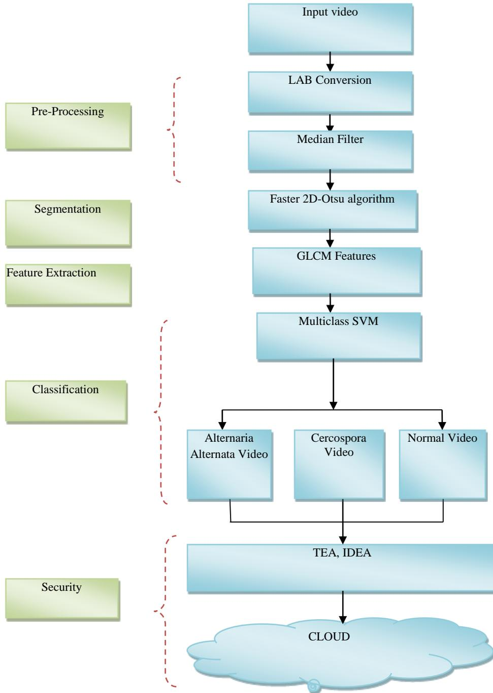
Figure 2: Proposed Flow Diagram
