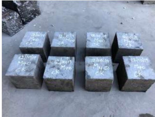
Figure 4: Test Specimens
