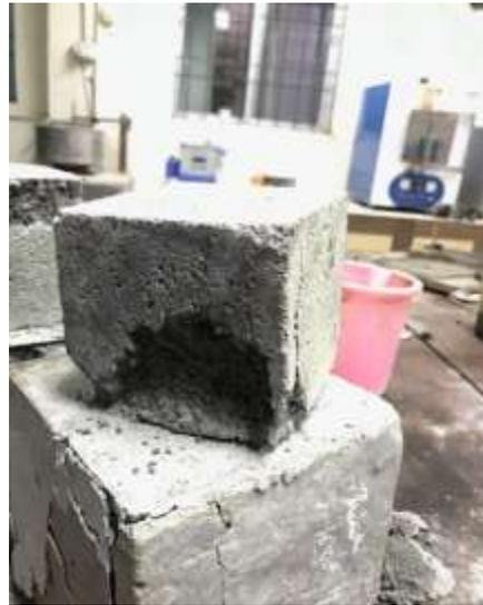
Figure 6: Specimen after Load Failure
