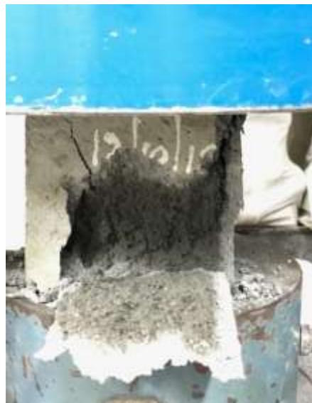
Figure 7: Air Bubbles Inside the Failed Specimen
