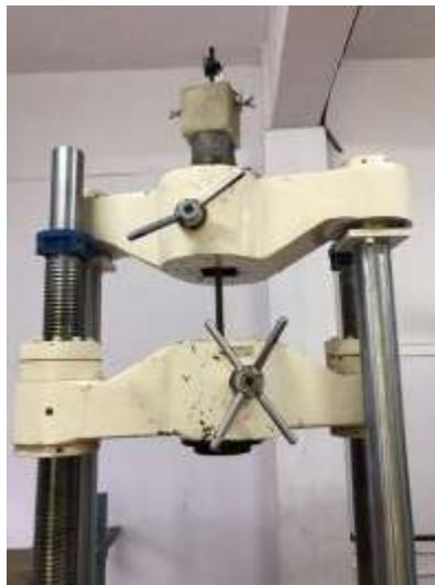
Figure 9: Specimen undergoing Pull out test
