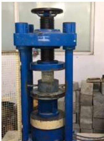
Figure 7: Specimen loaded in Compressive testing machine
