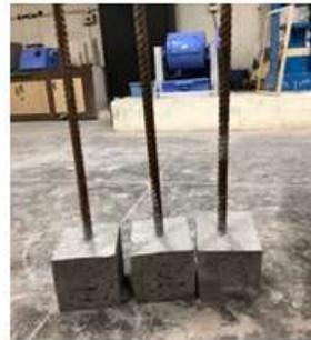
Figure 6: Pull out specimen
