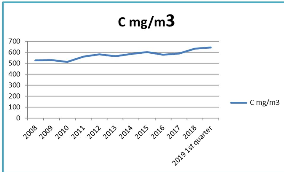
Figure 2: Concentration of Grain Dust before Cleaning in the Elevator
