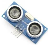
Fig. 1. Ultrasonic sensor
