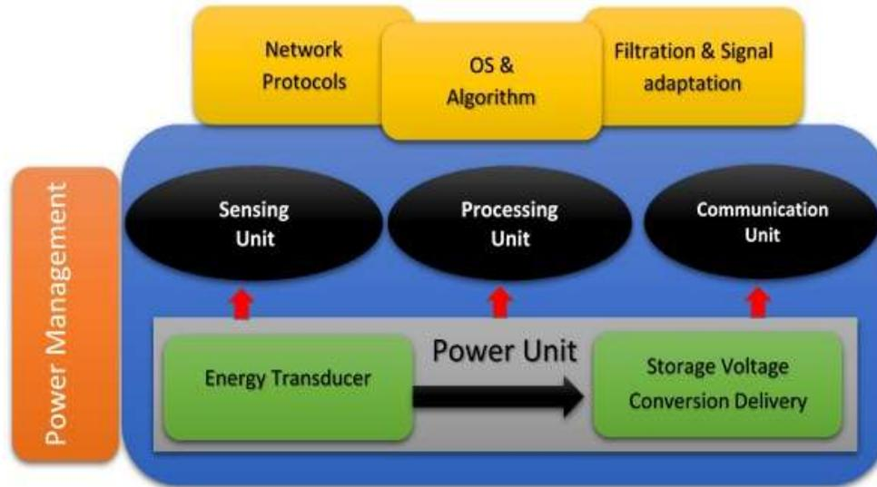
Fig. 1.1: Typical Sensor Node Architecture
