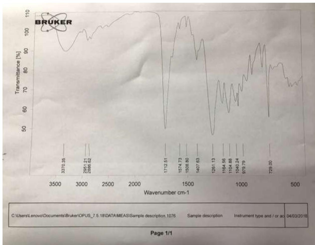
Figure 3: The FT-IR spectrum of graft co-polymer
