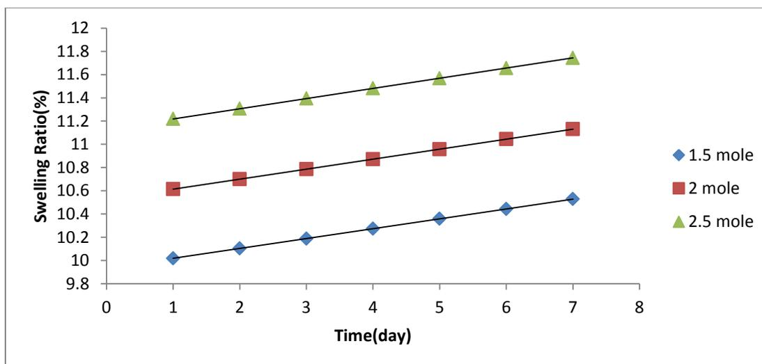
Figure 10: Swelling ratio (%) in day, of graft co-polymer with different moles of acrylic acid monomers in pH=8.0 at 310 K
