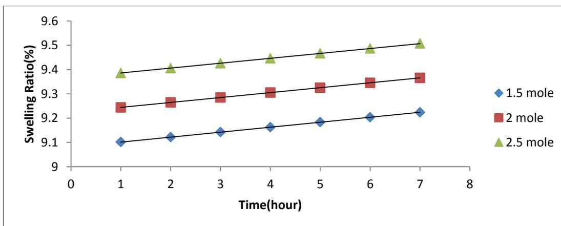
Figure 9: Swelling ratio (%) in hour, of graft co-polymer with different moles of acrylic acid monomers in pH=8.0 at 310 K
