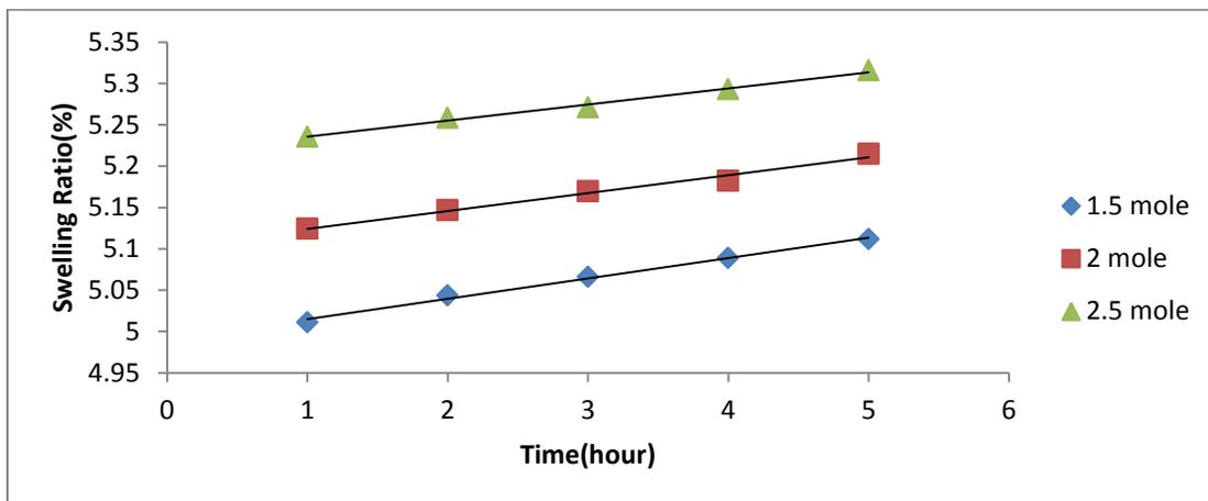
Figure 5: Swelling ratio (%) in hour, of graft co-polymer with different moles of acrylic acid monomers in pH=2.2 at 310 K
