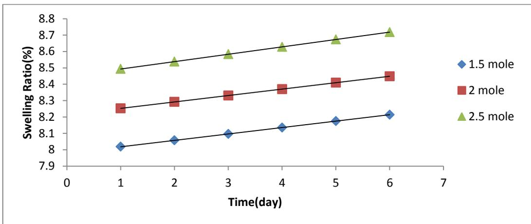
Figure 8: Swelling ratio (%) in day, of graft co-polymer with different moles of acrylic acid monomers in pH=7.0 at 310 K
