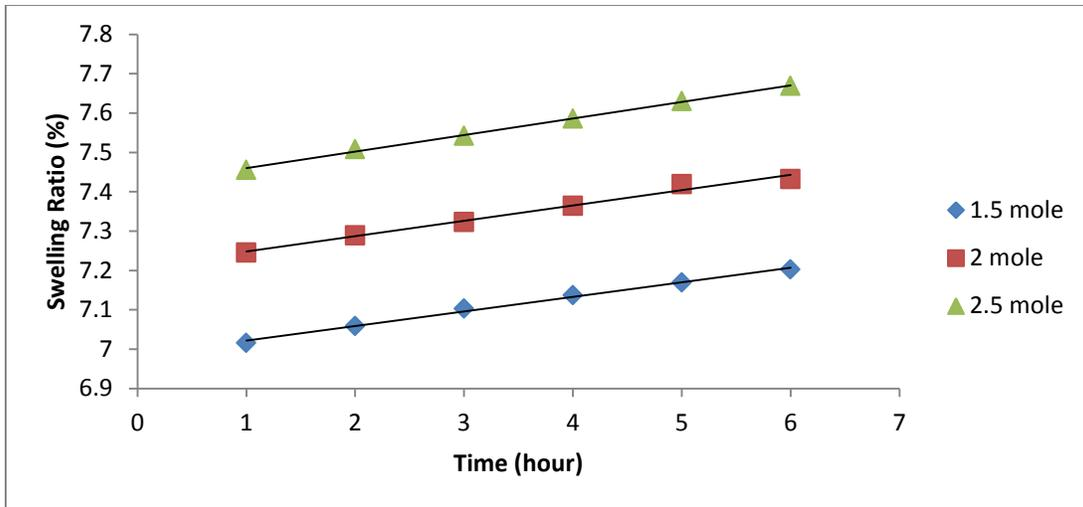
Figure 7: Swelling ratio (%) in hour, of graft co-polymer with different moles of acrylic acid monomers in pH=7.0 at 310 K
