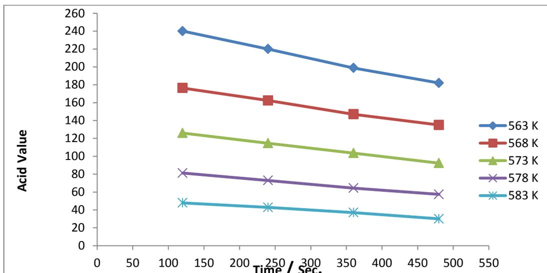
Figure 4: Acid value Vs. Time (Sec.) in different temperatures
