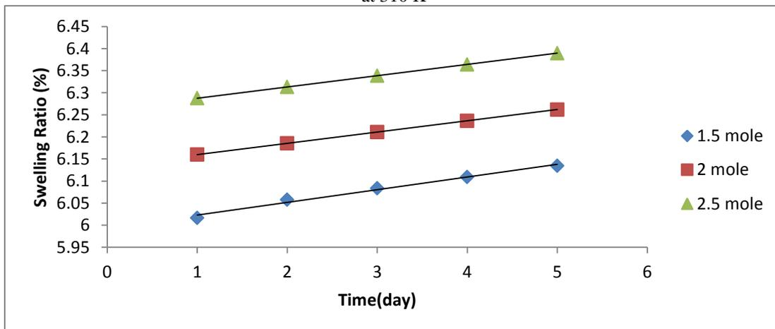
Figure 6: Swelling ratio (%) in day, of graft co-polymer with different moles of acrylic acid monomers in pH=2.2 at 310 K
