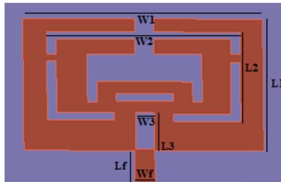
Fig. 1: Geometry for the Antenna
