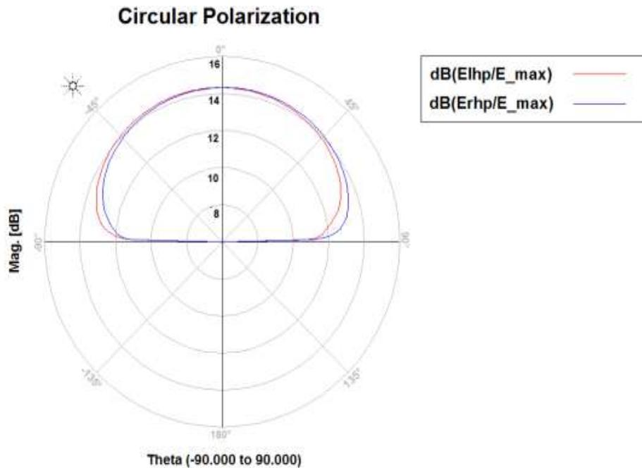
Fig. 21: Circular Polarization of Rectangular Patch Antenna Array
