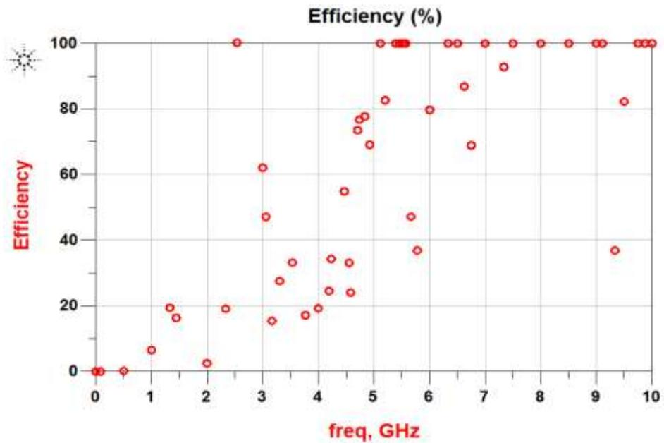
Fig. 7: Efficiency Vs Frequency of Rectangular Microstrip Patch Antenna
