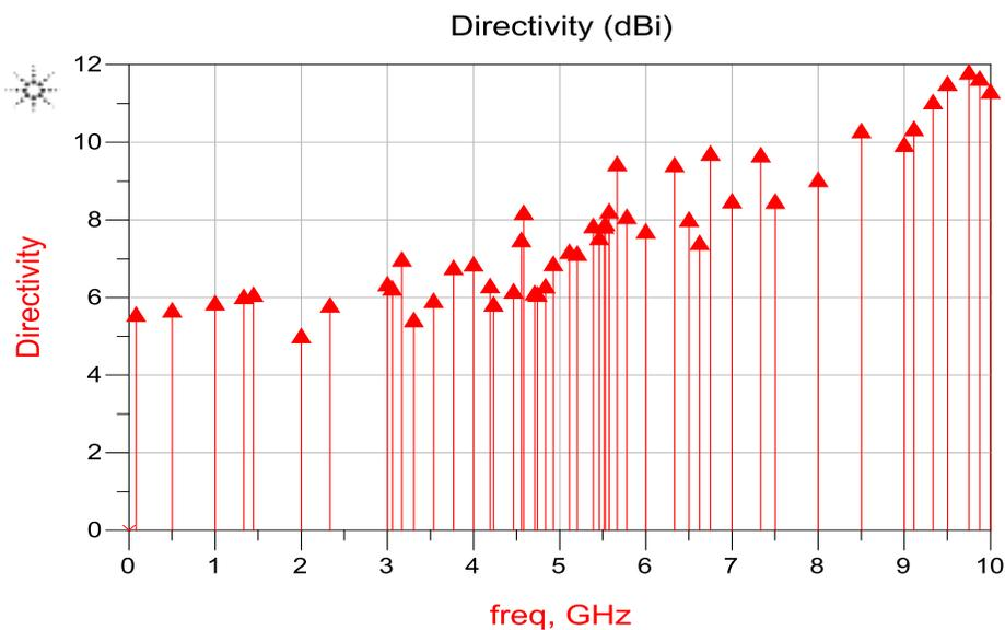
Fig. 6: Directivity Vs Frequency of Rectangular Microstrip Patch Antenna
