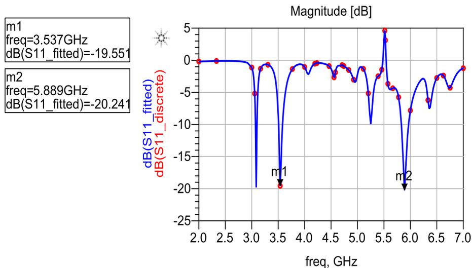
Fig. 4: Return Loss of Rectangular Microstrip Patch Antenna
