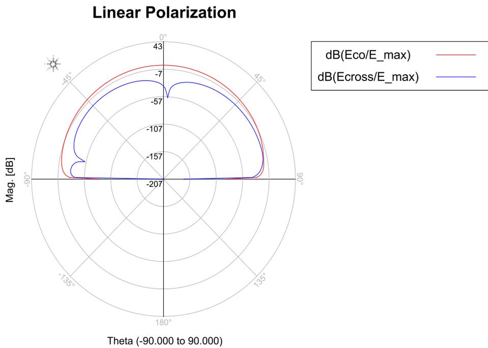
Fig. 10: Linear Polarization of Rectangular Patch Antenna
