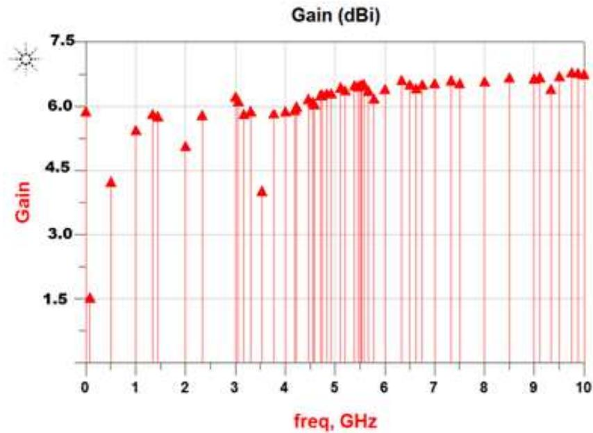
Fig. 5: Gain Vs Frequency of Rectangular Microstrip Patch Antenna
