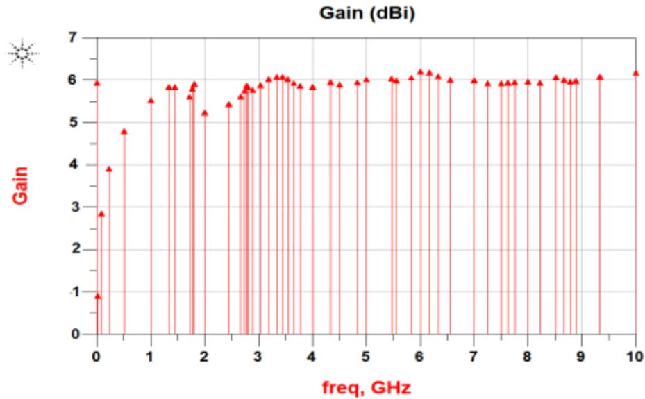
Fig. 15: Gain Vs Frequency of Rectangular Microstrip Patch Antenna Array
