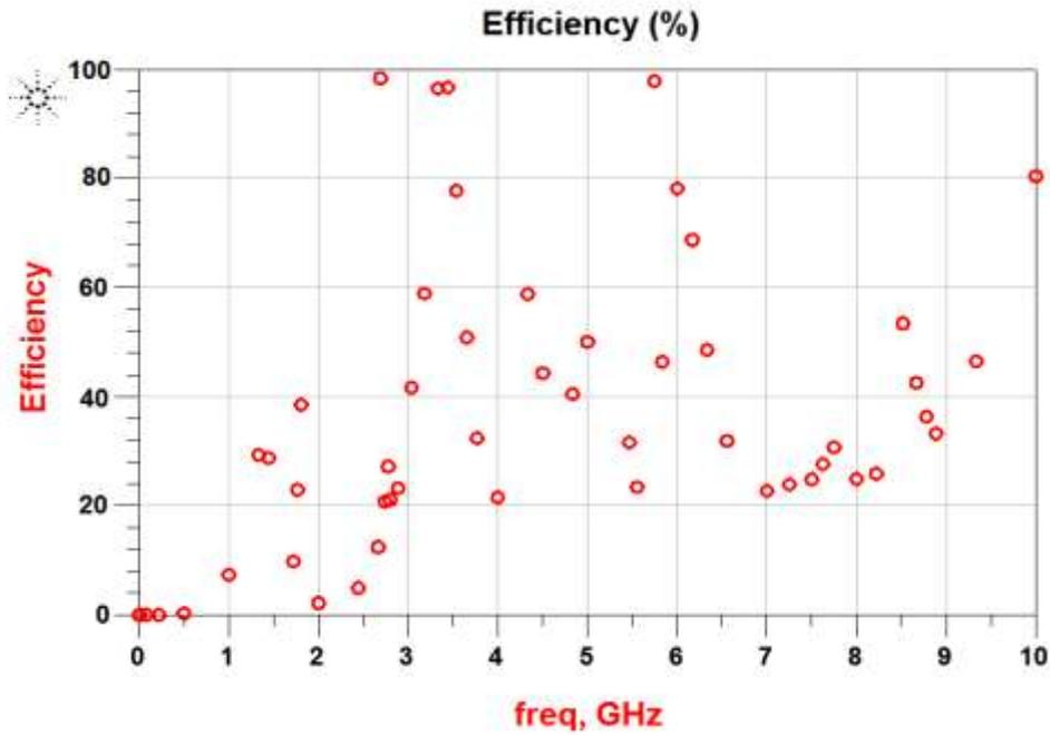
Fig. 17: Efficiency Vs Frequency of Rectangular Microstrip Patch Antenna Array
