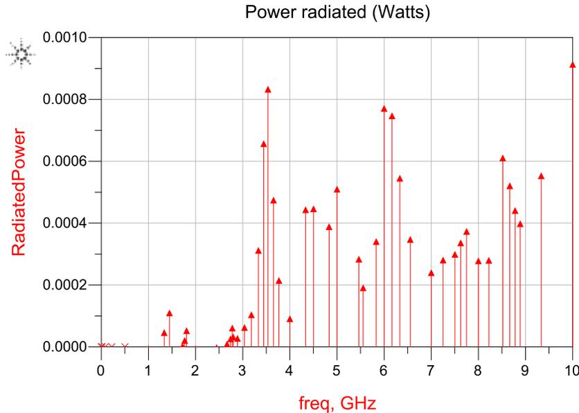
Fig. 8: Radiated Power Vs Frequency of Microstrip Patch Antenna
