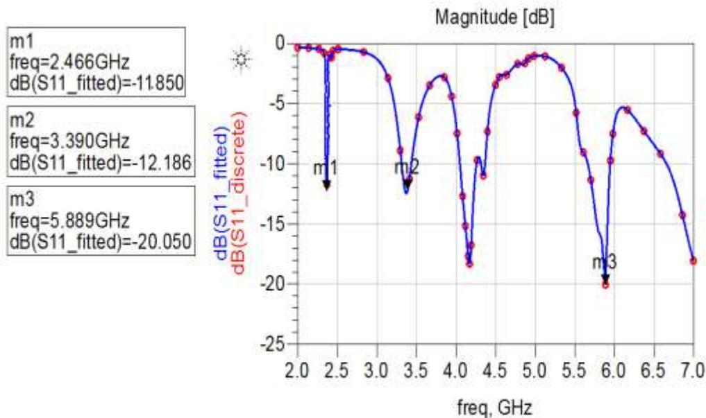
Fig. 14: Simulated Return Loss  $S_{11}$  of Antenna Array
