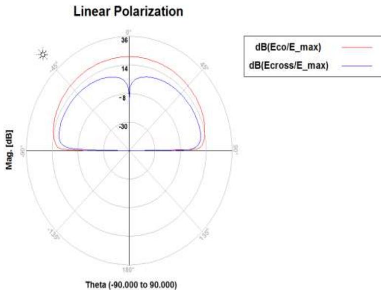
Fig. 20: Linear Polarization of Rectangular Patch Antenna Array
