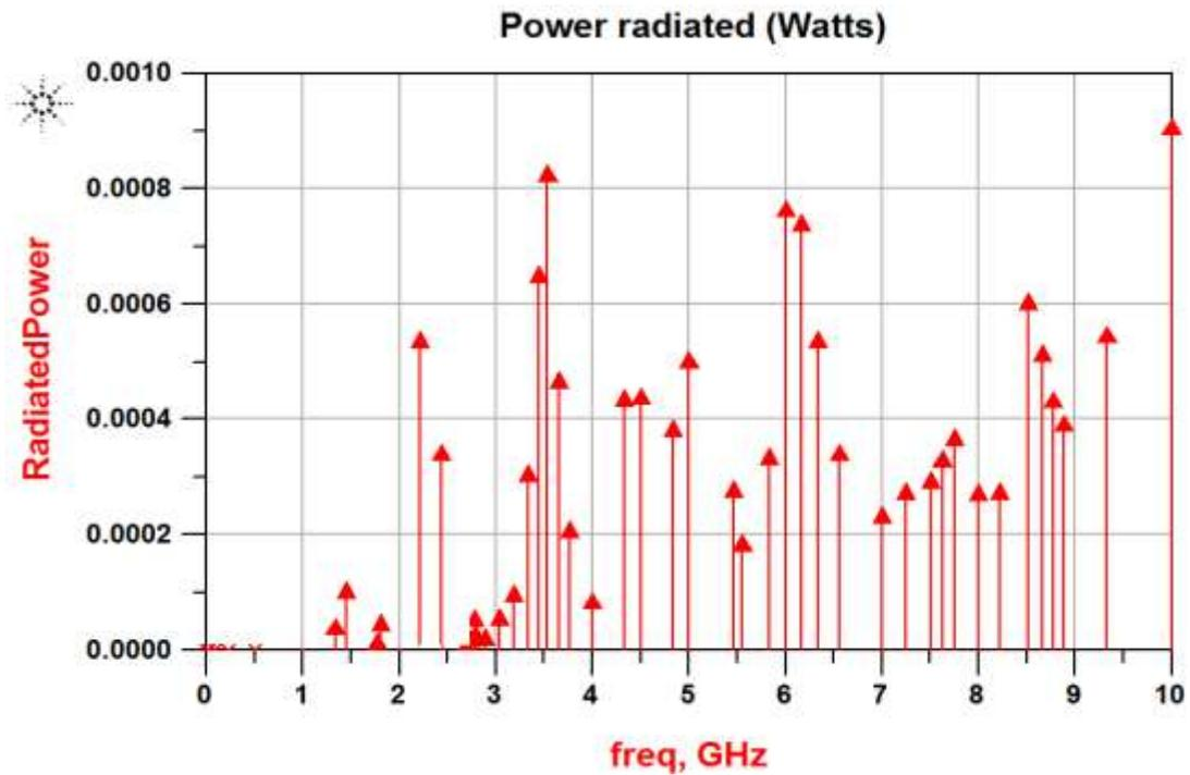
Fig. 18: Radiated Power Vs Frequency of Microstrip Patch Antenna Array
