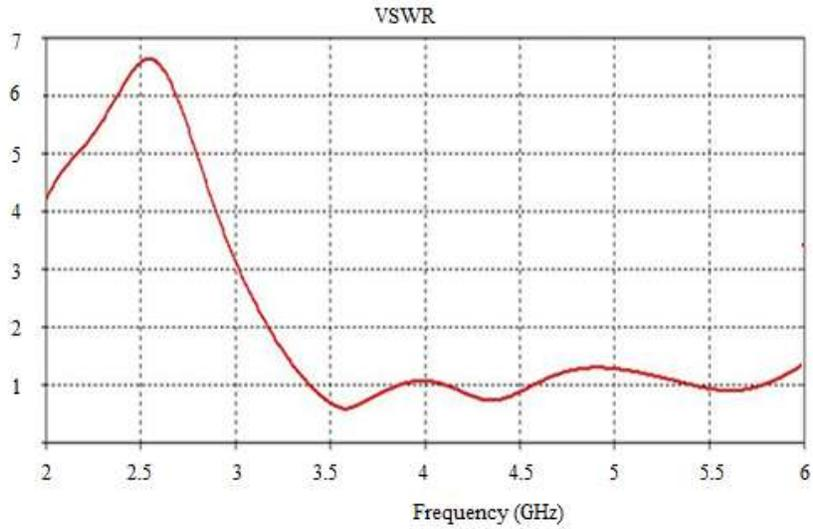
Fig. 9: VSWR Vs Frequency of Microstrip Patch Antenna
