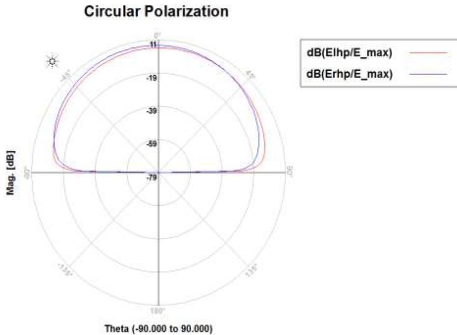
Fig. 11: Circular Polarization of Rectangular Patch Antenna
