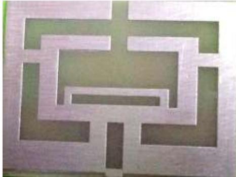
Fig. 3: Fabricated Single Antenna
