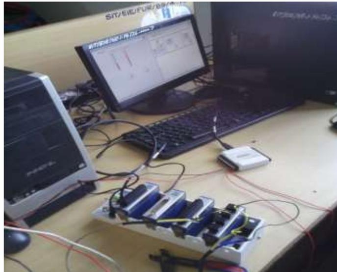
Fig. 6: Hardware setup of MHS interfaced with DAQ
