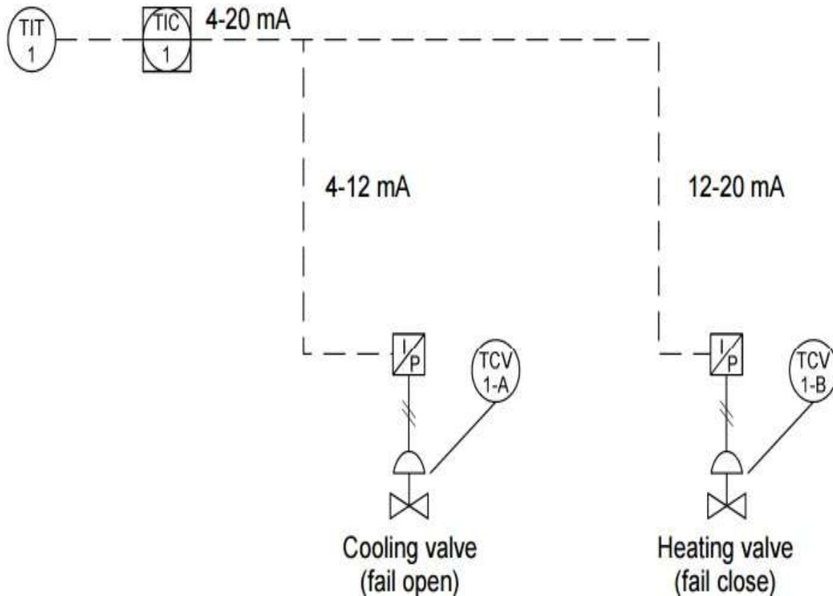
Fig. 7: Flow diagram of temperature process using SRC
