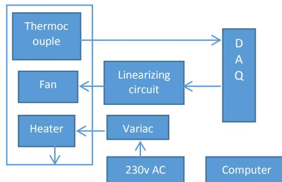
Fig. 1: Block diagram of MHS
