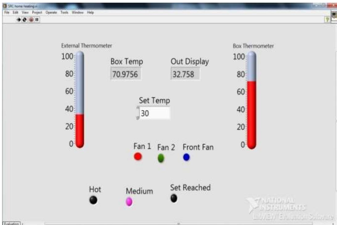
Fig. 11: Front Panel of MHC Setup in VI for Medium Condition
