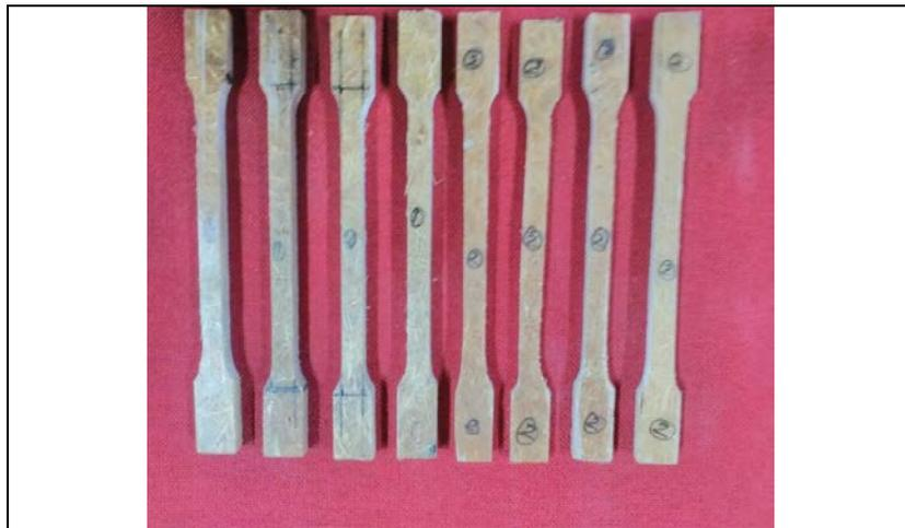
**Figure 7:**Untreated & alkaliized sisal fiber reinforced epoxy composite specimens as per ASTM D638
