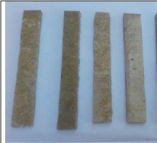
**Figure5:** Raw(Untreated) sisal fiber reinforced epoxy composite
