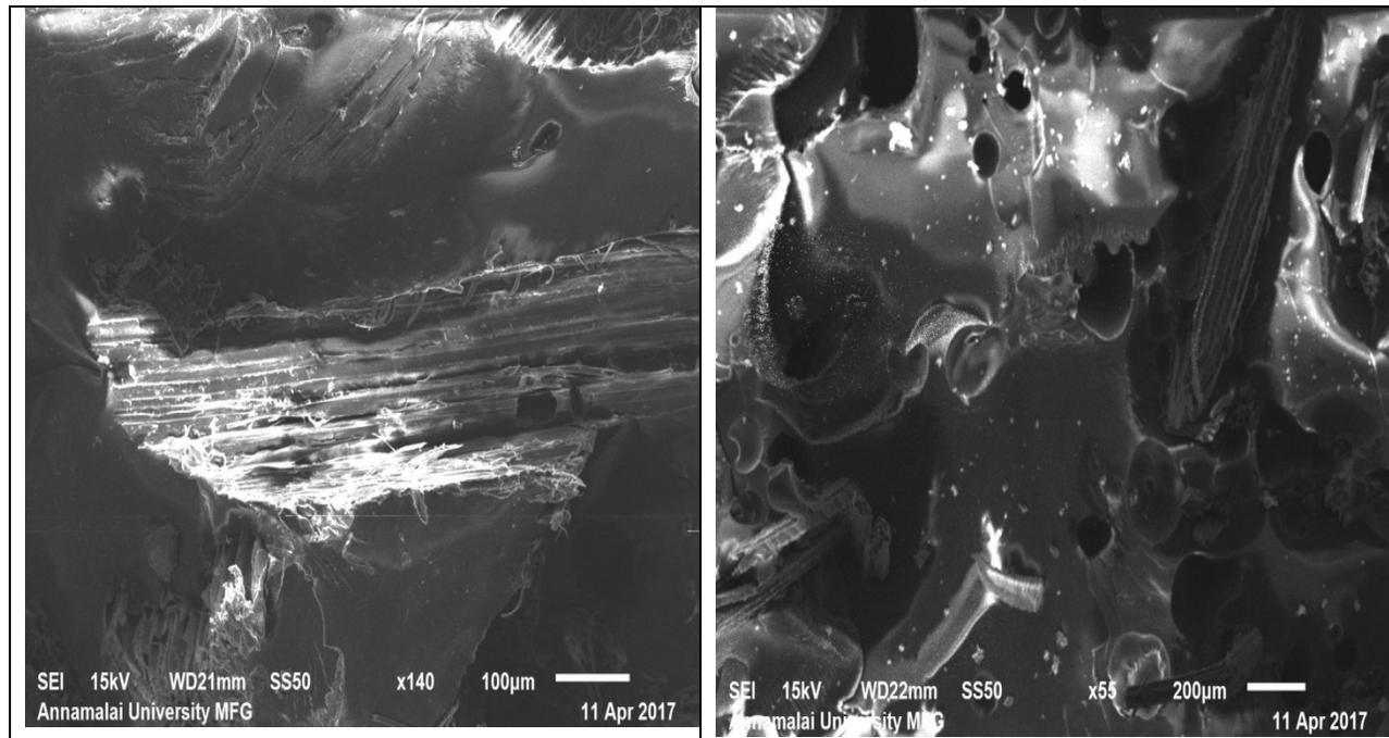
**Figure 10:**(a & b) The Micro-graph surface of Sodium hydroxide Treated Sisal fiber reinforced epoxy composite
