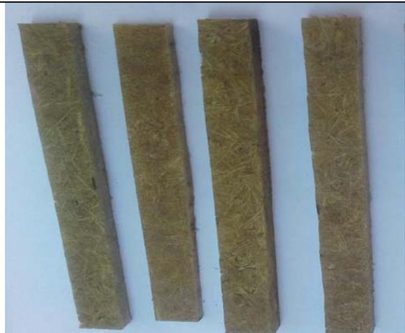
**Figure6:** Mercerized sisal fiber reinforced epoxy composite
