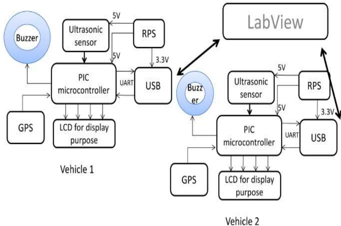
Fig.1 Block Diagram of Intelligence System for Potholes Detection Using LabVIEW
