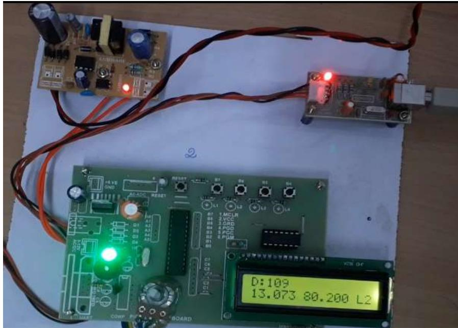
Fig 2 Hardware Implementation of Intelligence System for Potholes Detection Using LabVIEW
