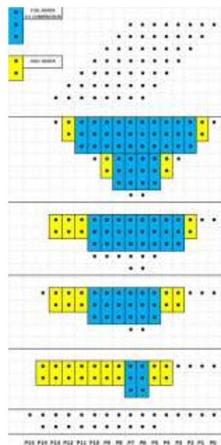
Fig. 7: Wallace Tree Multiplier using 3:2 Compressor
