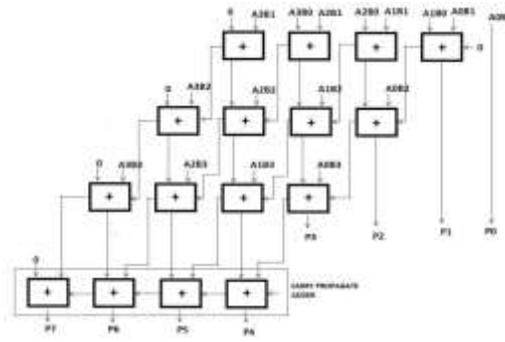
Fig. 6: Carry save Array Multiplier
