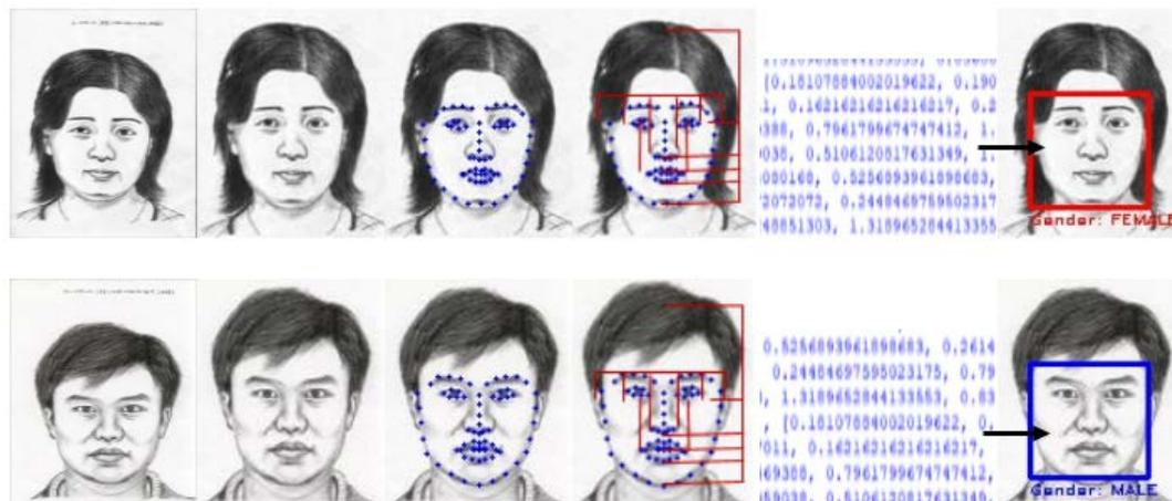
Figure 6: The process of our FSR, line1: extract of the dataset photos/input facial emotion. Line2: cropped emotional photos. line3: extract the 68 face landmarks points. Line 4: calculate of sixteen features and line5: the vector generated from the facial emotion photos, it is involved to Recognized the kind of Emotion. The output result of FER is the probe kind of Emotion of the Input Facial Photos
