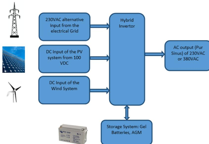
Fig. 1: Functional Diagram of the Adopted Hybrid Topology
