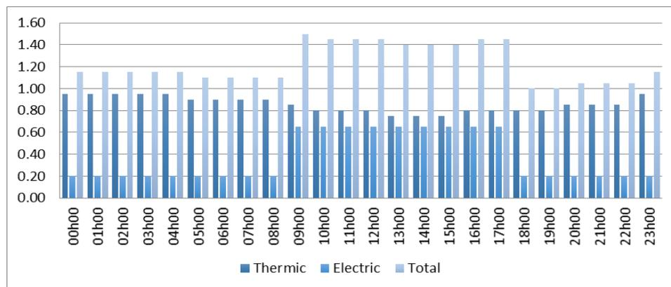
Figure 2: The Electric Load Profile of the Laboratory Prototype
