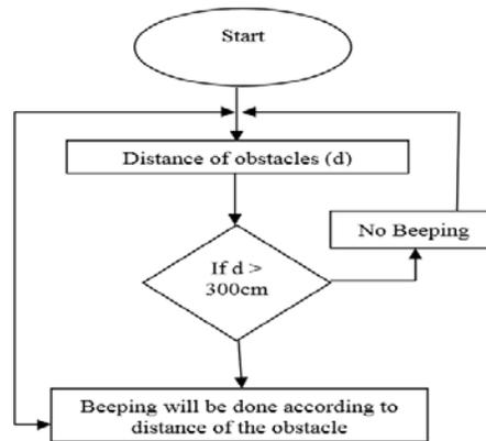
Fig 1: Flow chart for obstacle detection
