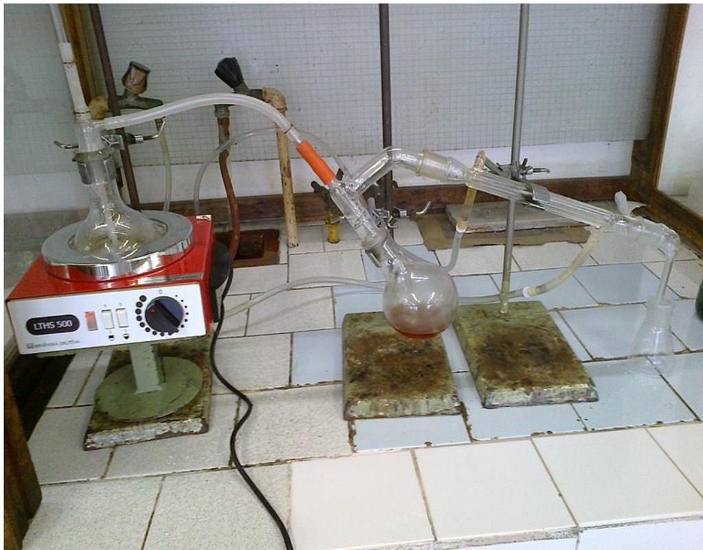
Apparatus for Steam Distillation
