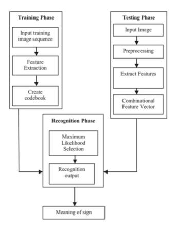
Fig. 2: Block diagram for the hand gesture recognition system
