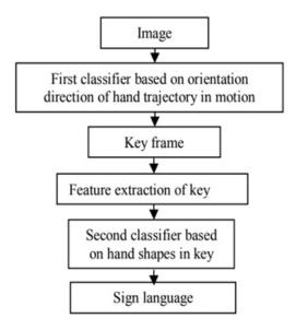
Figure 1: Flow diagram of proposed sign language recognition system
