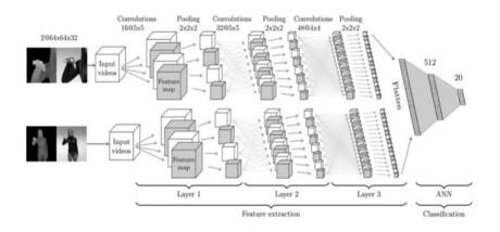
Fig .7: Architecture of CNN for sign language recognition system
