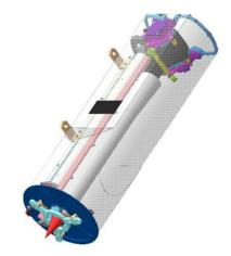
Fig.2: Reusable deep logging probe (RDLP).
