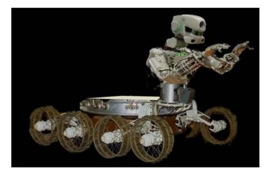
Fig. 14: The variant of the anthropomorphic robot of the Skybot f-850 project on a wheeled-walking chassis of moon rovers.
