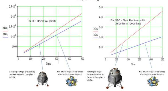
The dependence of the starting weight  $M_{pg}$  of the Ascent Descent Complex  $M_o$  by weight of the payload  $M_{n\sigma}$
