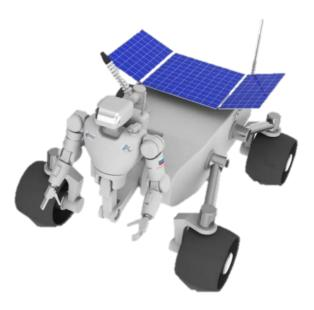
Fig.11:Lunokhod with the torso part of an anthropomorphic robot for research of stony, rocky rocks and with the possibility of repair (of itself and other lunar technology).
