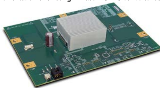
Fig. 6. System implementation of proposed new Bi-face DC-DC converter using single such board
