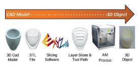
Generalized Additive Manufacturing Process.
