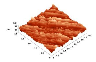
Fig 6.8: 5µm × 5µm 3D Image of Coated Sample At 600°C Temperature
