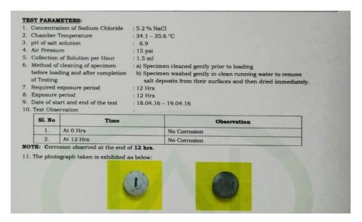
Fig 6.9: Salt Spray Test Results for Room Temperature Coated Sample
