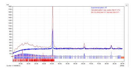
Fig 6.2: XRD - Results for Room Temperature Coated Piece
