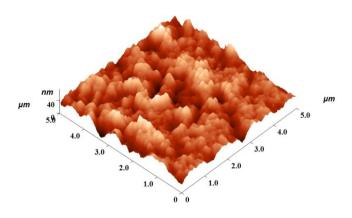
Fig 6.7: 5µm × 5µm 3D Image of Sample Coated At 400°C Temperature
