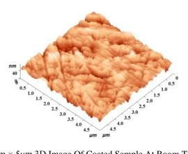
Fig 6.6: 5µm  $\times$  5µm 3D Image Of Coated Sample At Room Temperature
