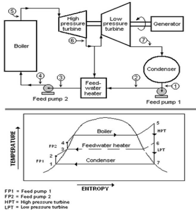
Fig.1: Feed water heater cycle
