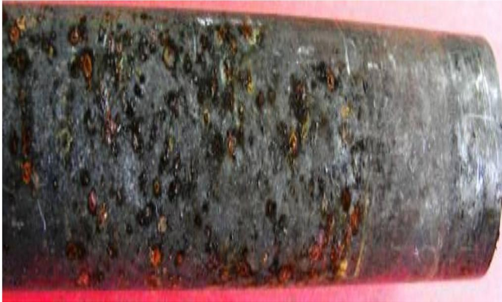
Fig.15: Degraded tube portion
