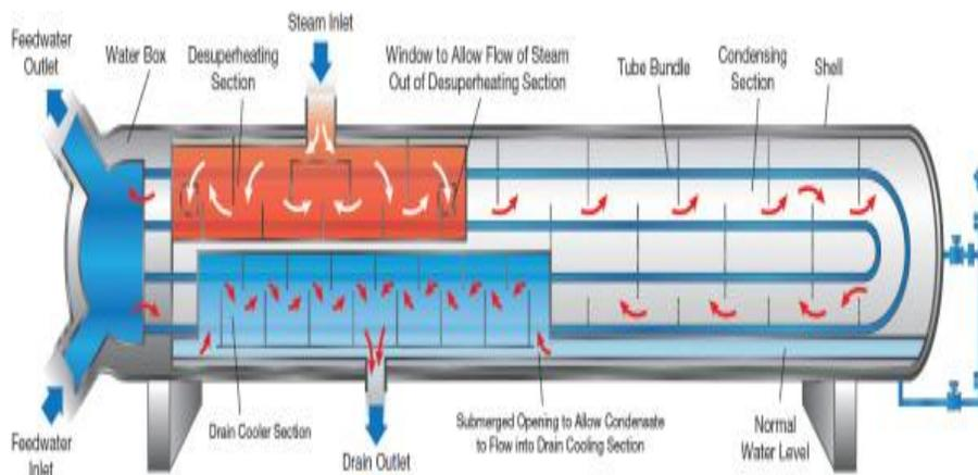
Fig.2: Different zones of Heater
