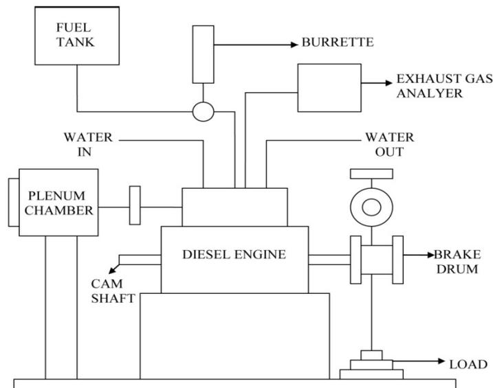
Schematic diagram of CI engine
