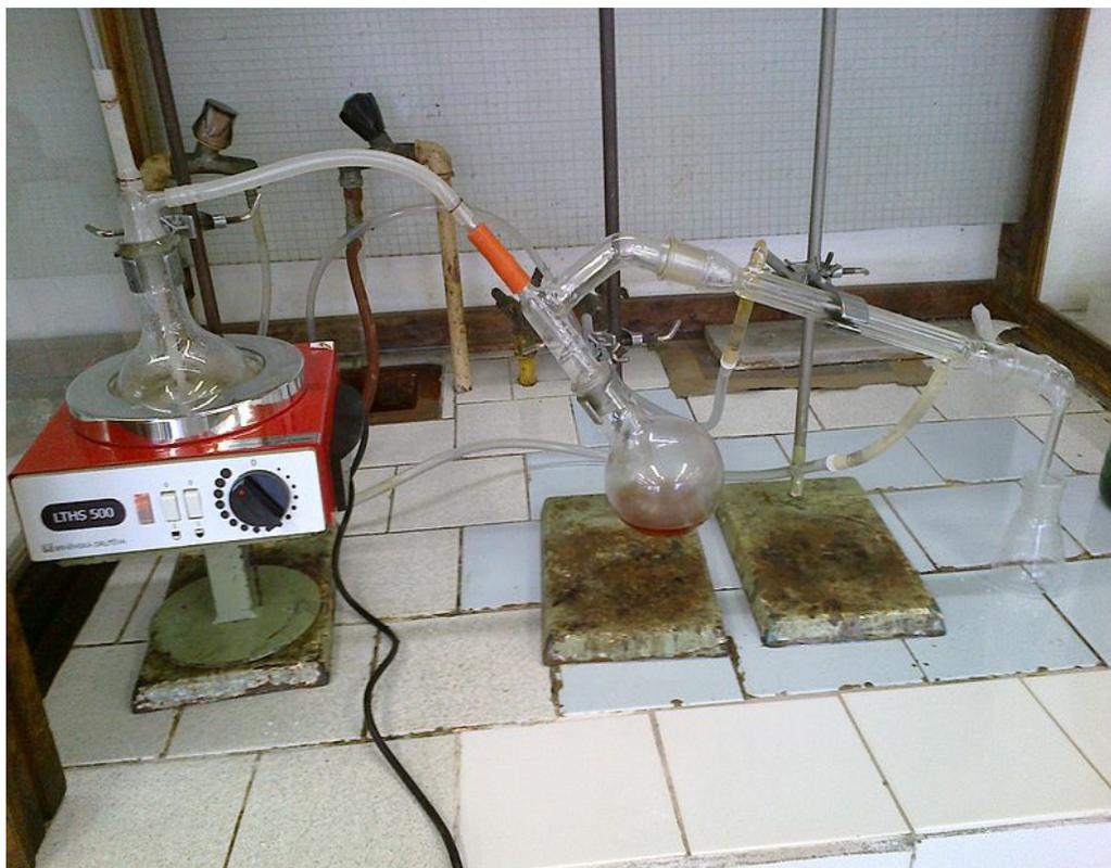
Apparatus for Steam Distillation
