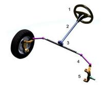
In this steering gear, a pinion is mounted at the end of the steering inner column. It engages the rack which has ball joints at each end to allow the rise and fall of the wheels, the rods are connected with ball joints to the sub axles. The rotary movement of steering wheel turn the pinion which moves the rock sideways parallel to tie rod.
