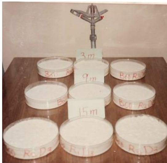
Figure 3. Containers of sieved wheat flour used in measuring sprinkler droplets.
