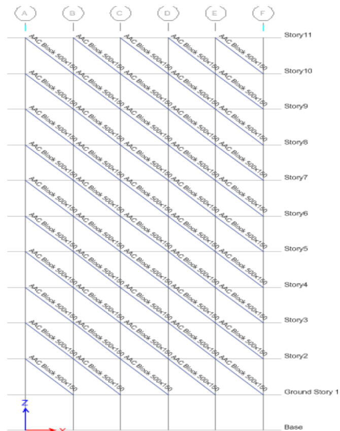
Fig.3.5 Elevation3D render view of building with AAC blocks as inclinedstruts
