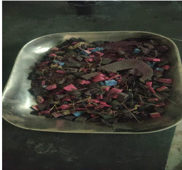
Figure 6.1- Making modified Bitumen by using Shredded footwear
