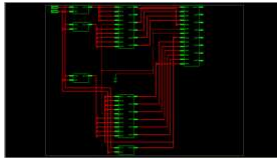
Figure 8 :RTL Schematic of QSD multiplier
