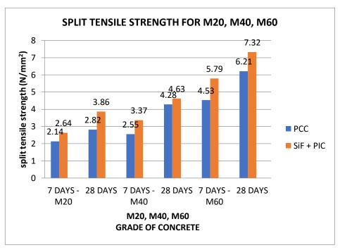
Figure 7 Comparison between silica fumes and conventional concrete
