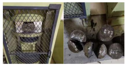
Fig 6 Figure Showing Split Tensile Strength
