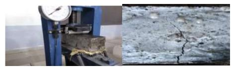
Figure 4 Showing Flexural Strength Of Concrete
