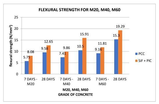
Figure 5 Comparison Between Silica Fumes And Conventional Concrete
