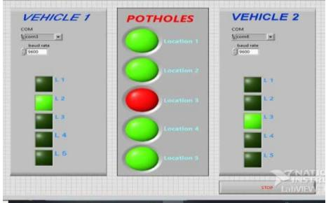
Fig 3 LabVIEW Front Panel of Intelligence System for Potholes Detection
