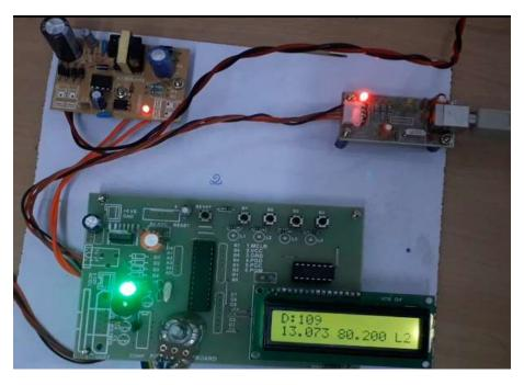
Fig 2 Hardware Implementation of Intelligence System for Potholes Detection Using LabVIEW
