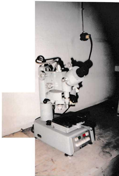
Fig. 4 Shimadzu Japan Microhardness Tester used to view the thickness of polyphenol layer
