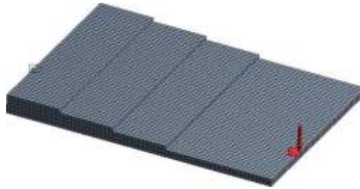
Fig 3.10: Stepped plate with solid elements
