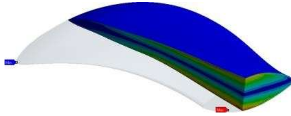
Fig. 7.9: Stress variation in composite blade
