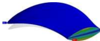
Fig. 7.8: Stresses in the composite blade
