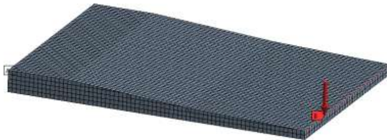
Fig. 3.11: Taper plate with Matrix elements after the ply dropoff.
