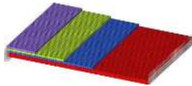
Fig. 3.6: Stepped plate with solid elements
