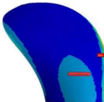
Fig. 4.1: Pressure distribution on suction side
