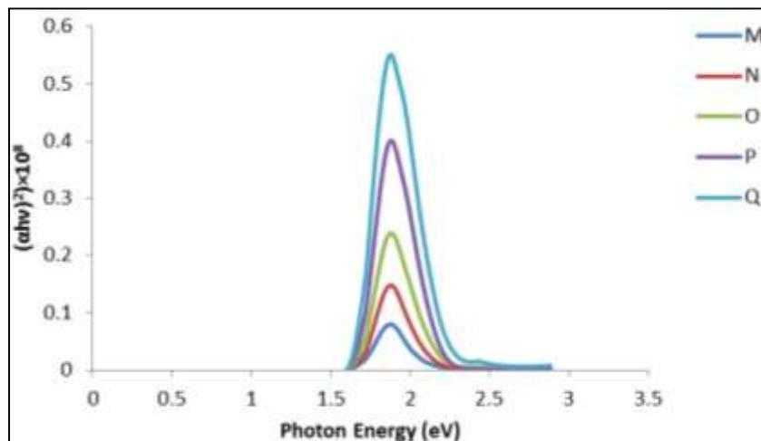
Figure 3: Relationship between  $(\alpha h\nu)^2$  and Photon Energy (eV) for (PEO/PVA) Composites Thin Films of different Concentrations of CoCl<sub>2</sub>.
