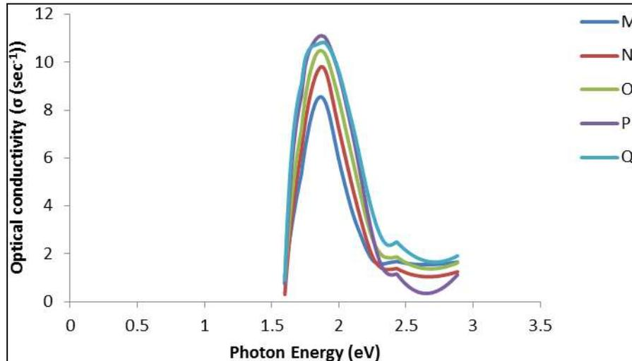
Figure 8: Optical conductivity as a feature of photon energy (eV) for (PEO/PVA) composites thin films of different concentrations of  $\text{CoCl}_2$ .
