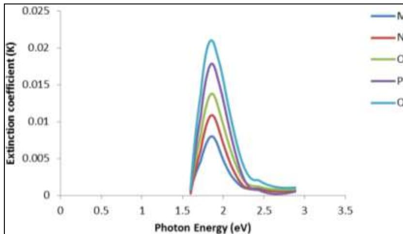
Figure 4: The variation of extinction coefficient with the Photon energy (eV) for (PEO/PVA) composites thin films of different concentrations of CoCl<sub>2</sub>.
