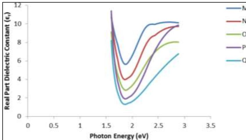
Figure 6: Real part dielectric constant against the Photon energy (eV) for (PEO/PVA) composites thin films of different concentrations of CoCl<sub>2</sub>.
