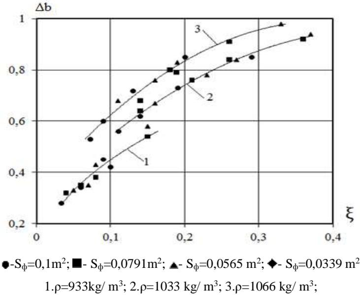
**Figure 5:** Correlation coefficient changes graph in depending on liquid velocity
