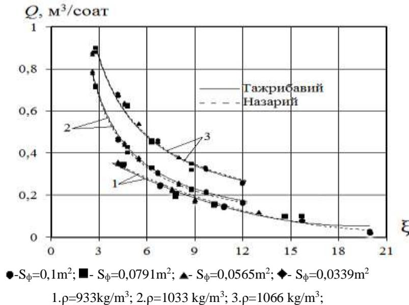
**Figure 4:** Fluid conductivity changes in depending on filter's resistance coefficient
