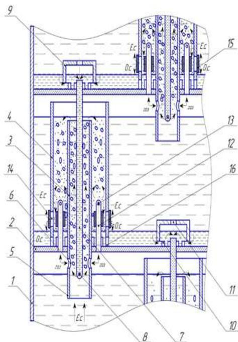
**Figure 1:** Scheme of bubble extractor
