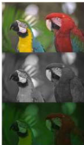
Fig. 3: Original image, 2D and 3D Bayer Array of Test Image
