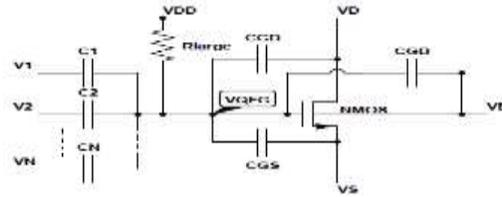
**Fig.2. Two-input QFGMOS transistor equivalent circuit**
