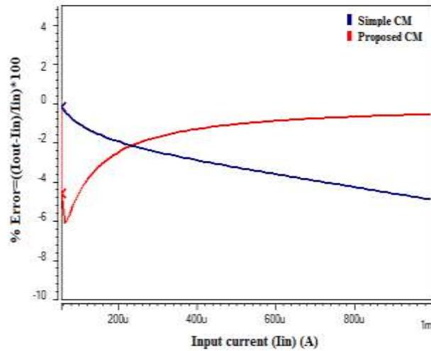
**Fig.6: Error in current transfer characteristics**
