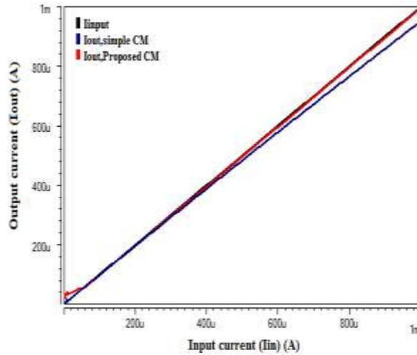
**Fig.5. Current transfer characteristics**
