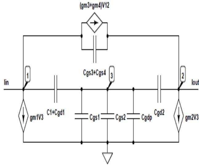
**Fig 4. High frequency model of Proposed CM**
