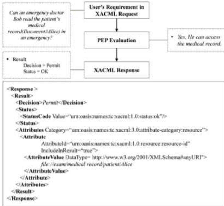
Fig. 5: An example of the method of generating AN XACML response message when analysis within the situation of Fig. 3.
