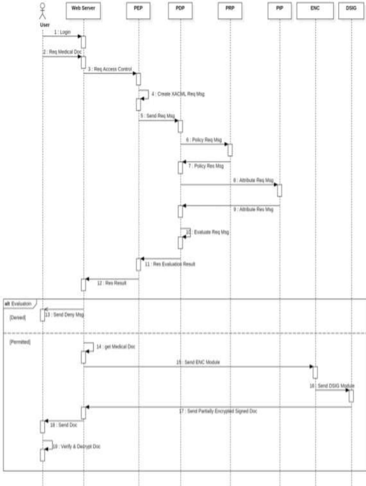
Fig. 8: The UML Sequence Diagram of the Implementation System.
