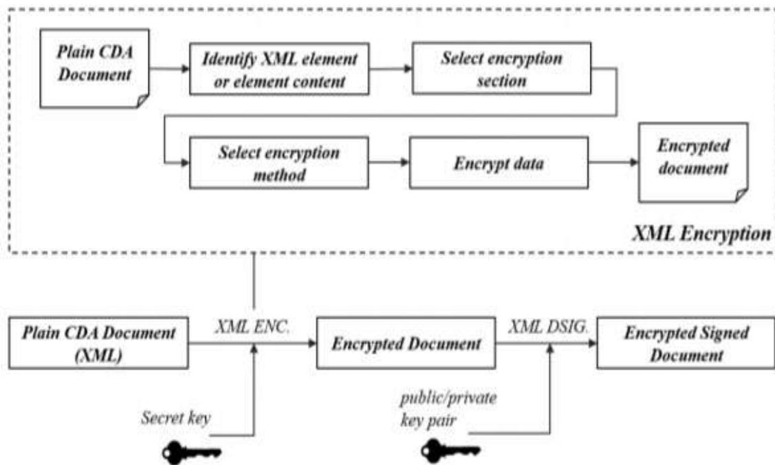
Fig. 6: The process of encrypting medical documents using XML encryption in phase 2 of the proposed model
