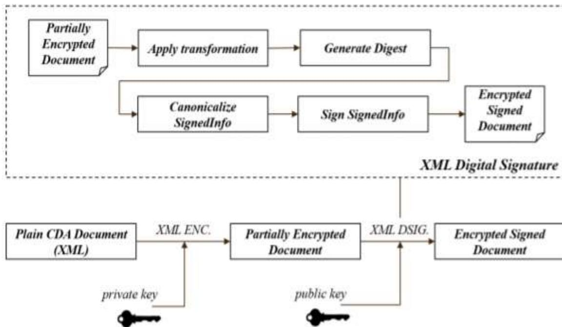
Fig. 7: The Method for Acting AN XML Digital Signature on a Partly Encrypted Medical Document in Fig. 6.
