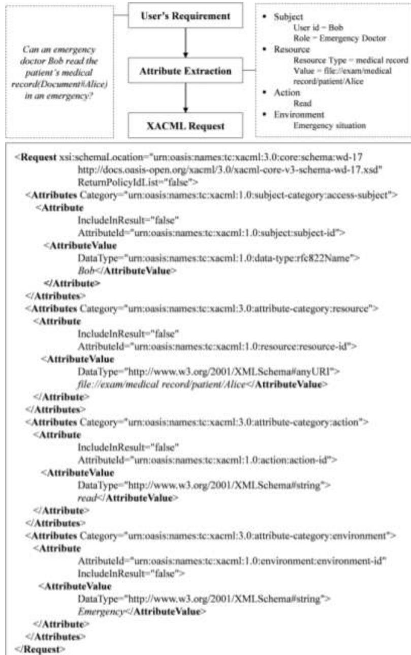
Fig. 3: An example of the method of generating AN XACML request message {in a |during a |in AN exceedingly| in a very} situation wherever the emergency doctor Bob accesses patient Alice's information in an emergency
