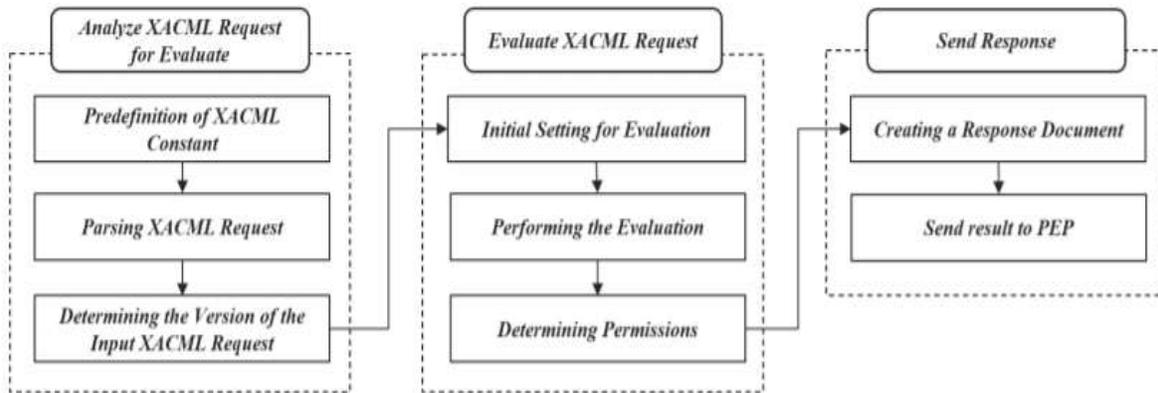
Fig. 4: The process of analyzing the request message and performing the evaluation process by the PDP to determine whether the user is a user who can access the patient's document
