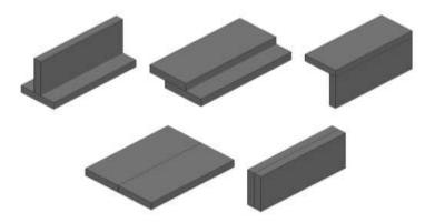
Figure 3: Image 3D Model Type of Welding Joints
