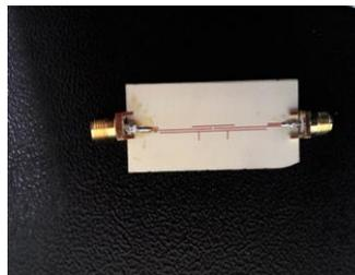
**Figure 9:** The filter after fabrication
