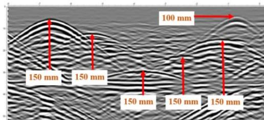
**Figure 8:** The radargram that represent the subsurface of the test base
