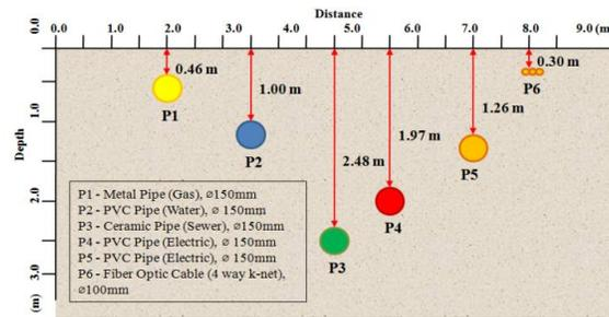
**Figure 6:** Test base in cross-section view
