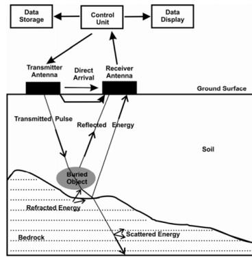
**Figure 4:** The GPR Principle [27]
