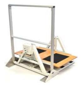
Figure 1: Lafayette Stability Platform with Digital Control Model 16030SR
