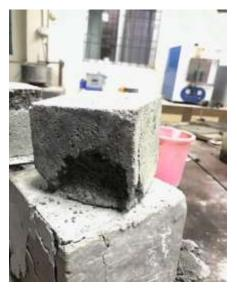
Figure 6: Specimen after Load Failure
